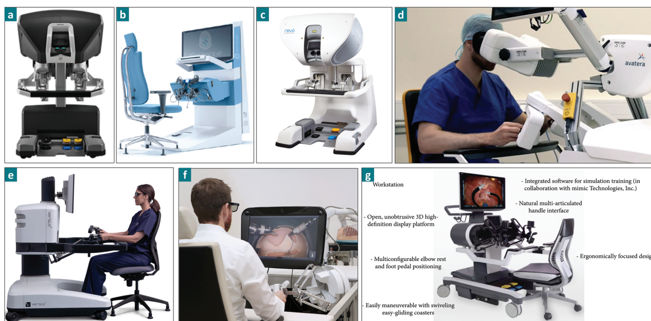
Figure 2. Master consoles or user interfaces of the laparoscopic surgical systems: a) DaVinci system (Intuitive Surgical, Inc.). Reproduced with permission. [41] Copyright 2022, Intuitive Surgical, Inc.; b) Senhance surgical system (Asensus Surgical Inc.). Adapted with permission. [13] Copyright 201, MDPI; c) REVO-I surgical robot system (meere company). Reproduced with permission. [42] Copyright 2021, revo; d) Avatera surgical robot system (Avateramedical GmbH). Adapted with permission. [43] Copyright 2022, avateramedical GmbH; e) Versius surgical system (CMR surgical Ltd.). Reproduced with permission. [44] Copyright 2022, CMR Surgical Ltd.; f) MiroSurge system. Reproduced with permission. [26] Copyright 2021, Springer Nature; g) Enos system (Titan Medical Inc.). Reproduced with permission. [46] Copyright 2021, Hindawi.
