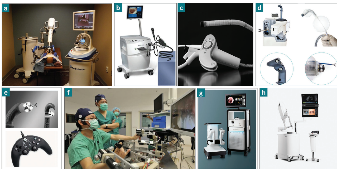
Figure 3. Master consoles or user interfaces of the endoscopic surgical systems: a) Flex Robotic System (Medrobotics Corp., Massachusetts, USA). Reproduced with permission. [66] Copyright 2022, Springer Nature; b) NeoGuide system (NeoGuide Endoscopy System Inc., Los Gatos, CA USA). Adapted with permission. [53] Copyright 2019, John Wiley and Sons; c) Invendoscope SC210 (Invendo Medical GmbH, Weinheim, Germany). Adapted with permission. [67] Copyright 2021, Springer Nature; d) Aer-O-Scope system (GI View Ltd., Ramat Gan, Israel). Adapted with permission. [53] Copyright 2019, John Wiley and Sons; e) Endotics system (ERA Endoscopy Srl, Pisa, Italy). Adapted with permission. [53] Copyright 2019, John Wiley and Sons; f) EndoMaster EASE system (EndoMaster Pte., Ltd., Singapore). Reproduced with permission. [68] Copyright 2017, arXiv. g) Monarch platform (Auris Surgical Robotics, Silicon Valley, CA, USA). Reproduced with permission. [69] Copyright 2021, MDPI.; h) Ion endoluminal system (Intuitive Surgical, Inc., Sunnyvale, CA). Reproduced with permission. [41] Copyright 2022, Intuitive Surgical, Inc.
